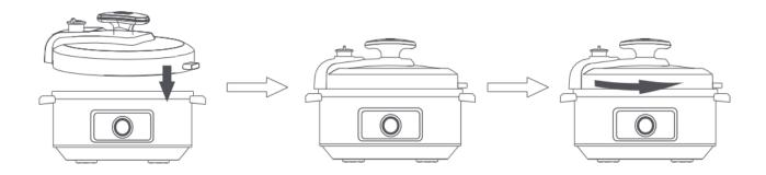
6. Check whether the float valve has been installed, and switch on the power supply.
