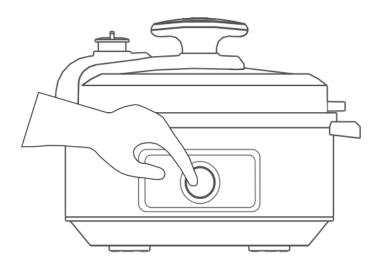
8. When the food is cooked, unplug the power plug. After the cooker cools down, check the float value falls completely. Then hold on the handle and open the lid.
