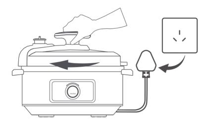
9. Before opening the lid, press the pressure release button by hand. When pressing the exhaust button, keep the angle of your hand to exhaust port between 90° and 270°, to prevent steam scald. Only when float valve falls completely, can you open the lid.
